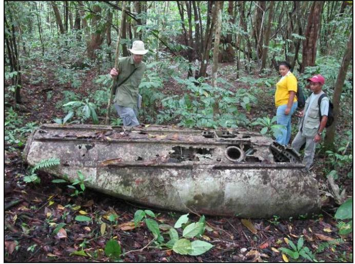
**Figure 5.24** Two views of an aluminum sea plane float, tentatively identified as Japanese.
