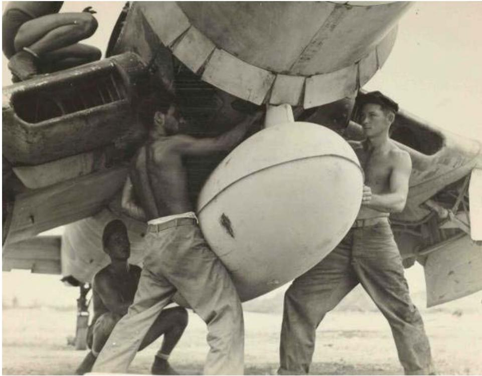
**Figure 7.53** American ground crews attach belly tanks full of napalm to Corsairs at Peleliu airfield in 1944. (NARA; RG127)
