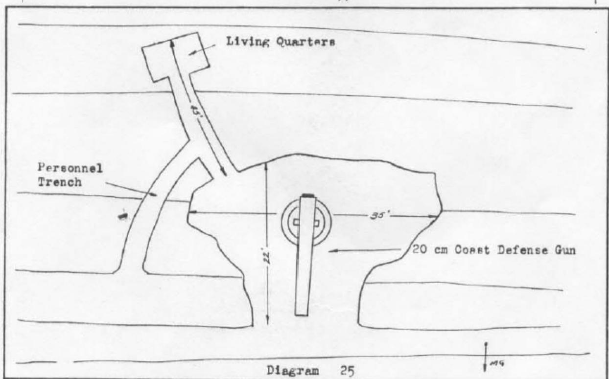
**Figure 6.17** War era sketch of the gun emplacement at site AB133 (after Phelan 1944)
