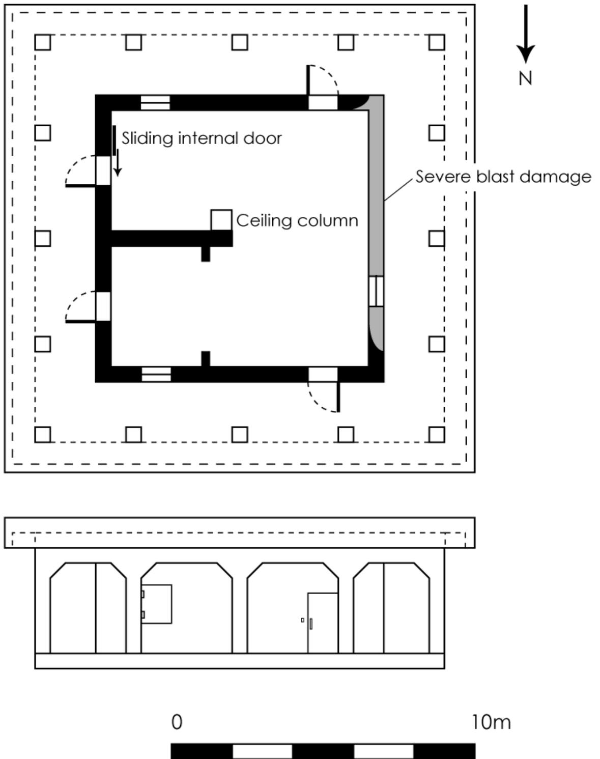
**Figure 5.64** Plan view of the Japanese Airfield Operations Building, AB262. (Drawing by Gavin Lindsay)
