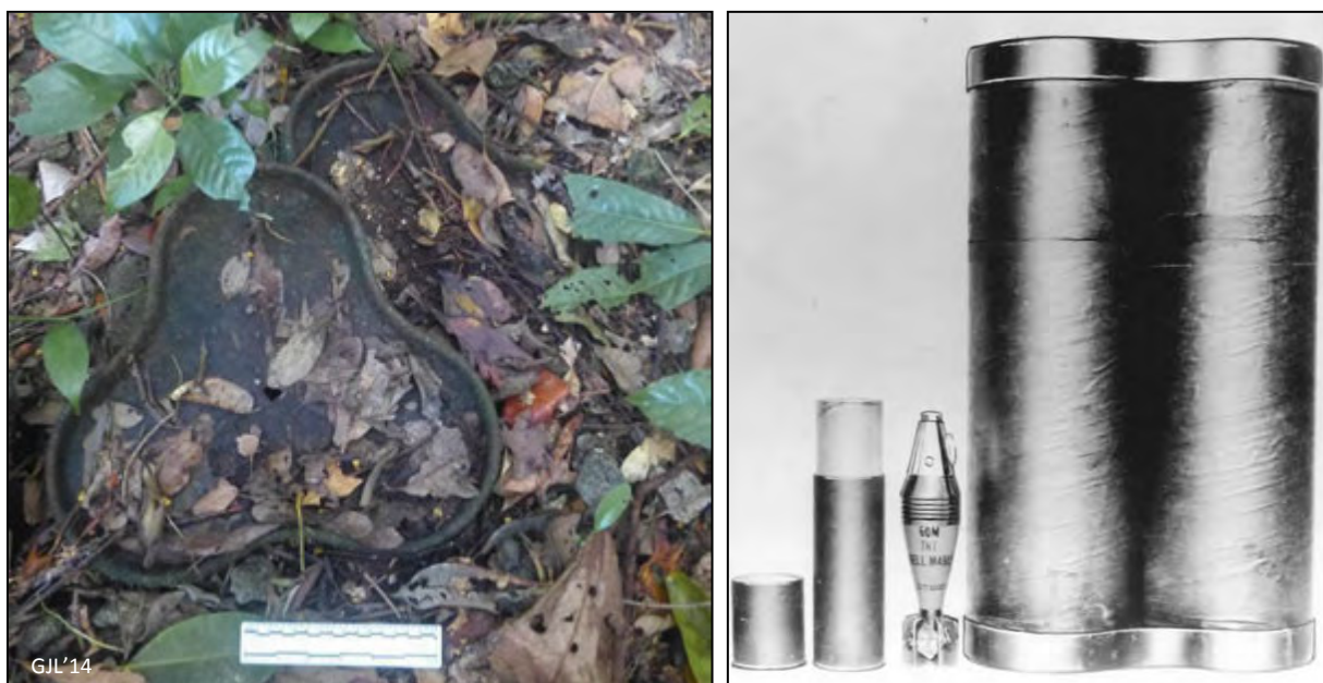
Figure 135 - AB14-SF066: 60mm mortar bomb '18 to bundle' cloverleaf ammunition containers
