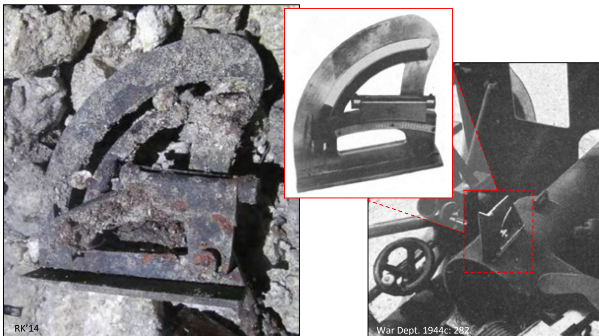
Figure 117 - AB14-059: gunners quadrant, calibrated from 0° to 90°. Relative mounting position on 75mm field gun shown on right
