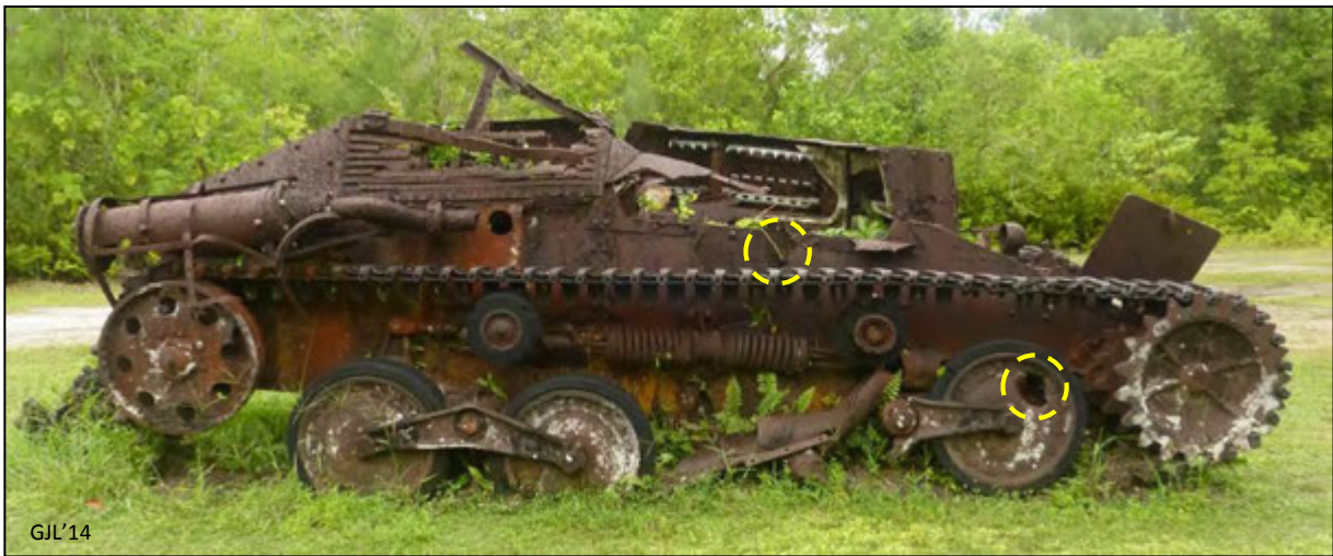
Figure 178 - AB141: IJA Type 95 Ha-Go Light Tank showing projectile impacts on starboard side
