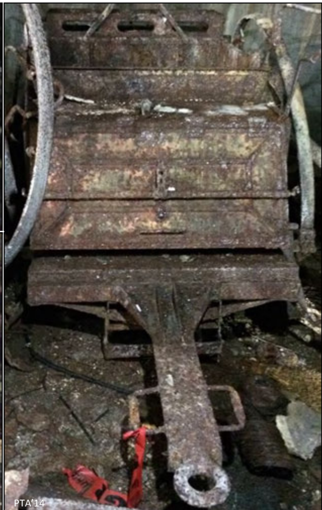
Figure 183 - AB14-111: Battery wagon (right) and limber, showing square storage detail
