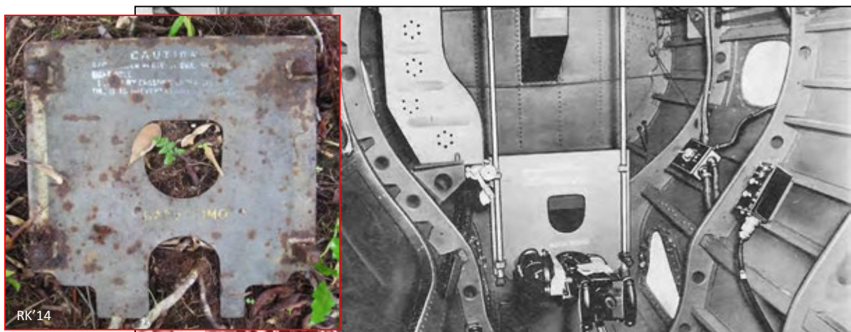
Figure 27 - Sliding armor plate for ventral gun in Bombardiers compartment at AB14-003B
